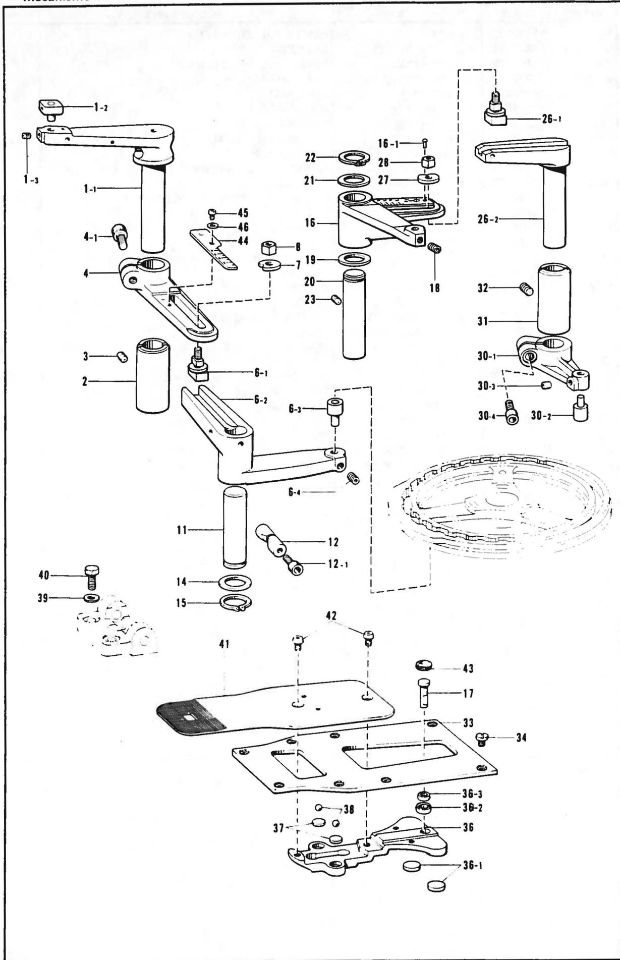
E. 送り関係/Feed mechanism/Transportvorrichtung/
