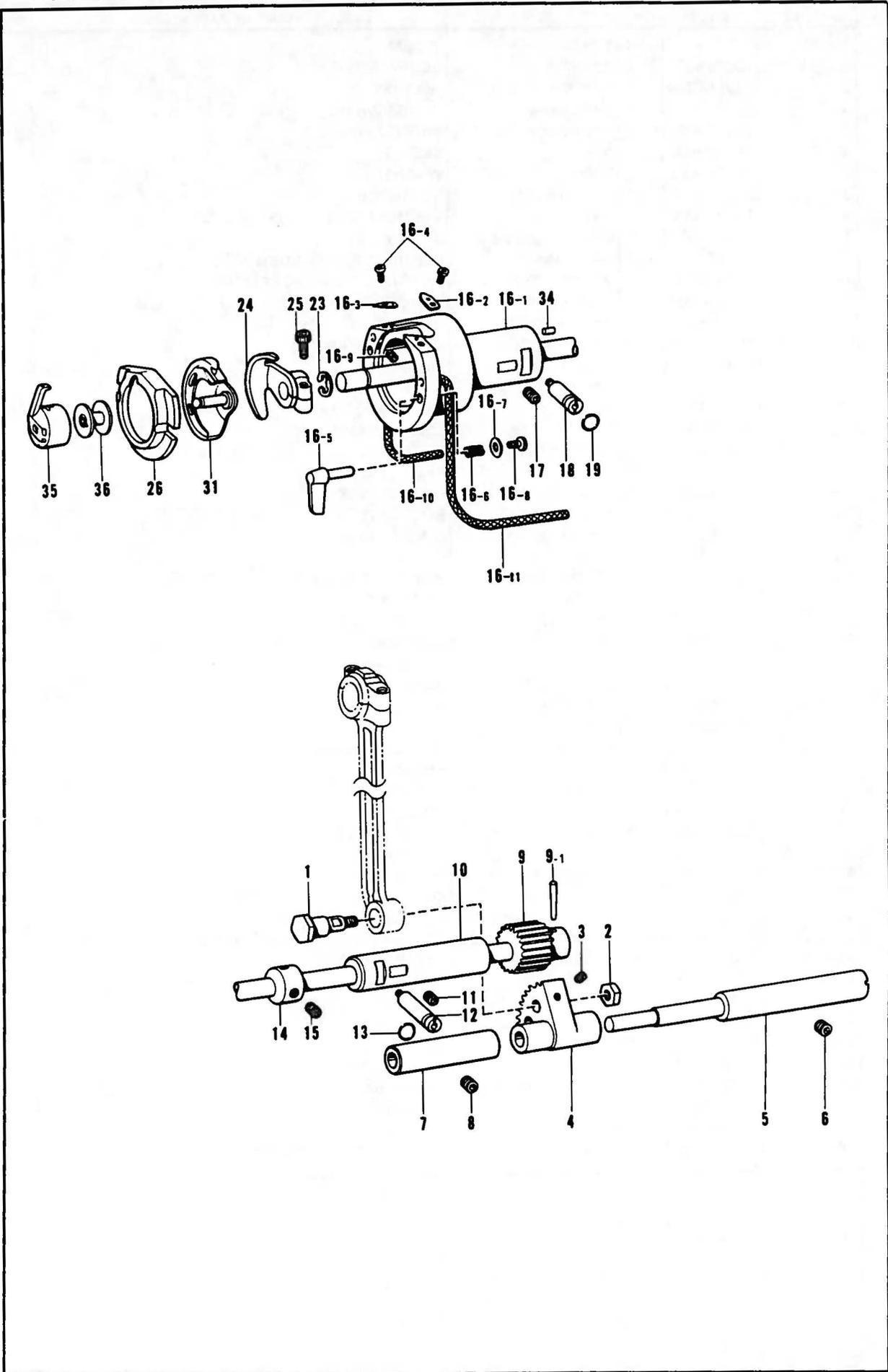
J. 下軸関係 / Lower shaft mechanism / Untere Welle
